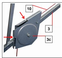
➤ Place the wire rope (10) in the grooves of both rope pulleys (3c).
