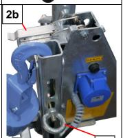
To remove the chassis, open the clamp lock (2b) and pull out the transportation frame (1).
