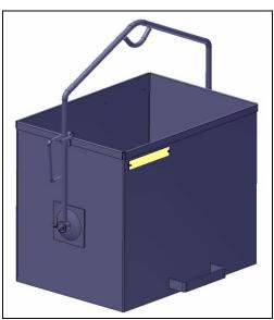
> To tip out, open the safety device (2) and tilt bucket (1).
