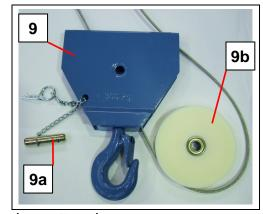
> Secure locking pin (9a) with the spring cotter pin.
