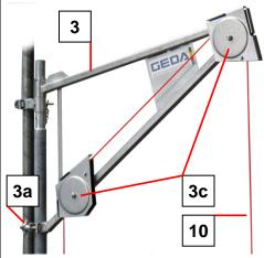
➤ Release the pivot arm locking device, swivel the pivot arm (3) outwards and tighten the star handle (3a).
