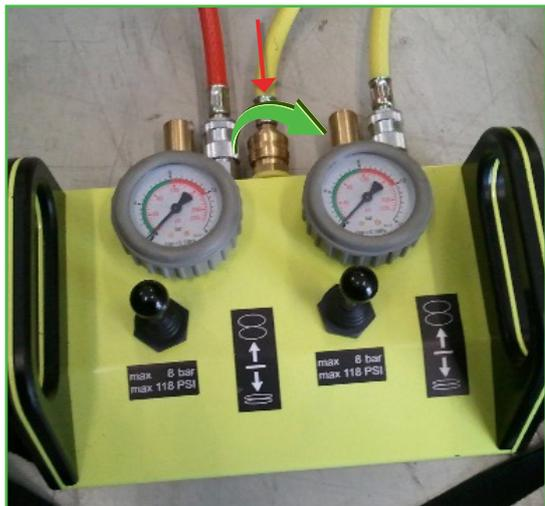
Connect the hose connector to the inlet air supply coupling on the controller, see the arrow in Fig. 5.8. If correctly inserted, the coupling on the controller clicks into place. Move the coupling housing by 180° left or right to lock the coupling.
