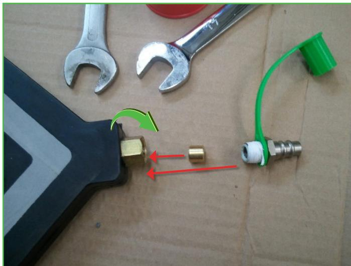
Fig. 6.3: Attaching a new connector
