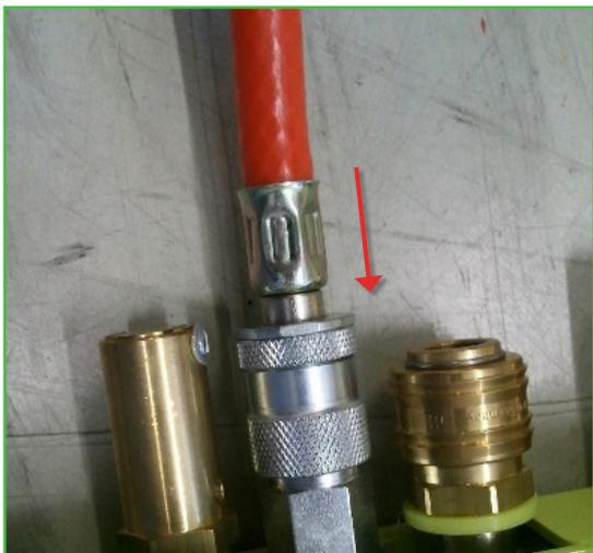
Connect the hose from the lifting bag to the connection coupling on the controller, see Fig. 5.4. If inserted correctly, the connection coupling clicks into place.
