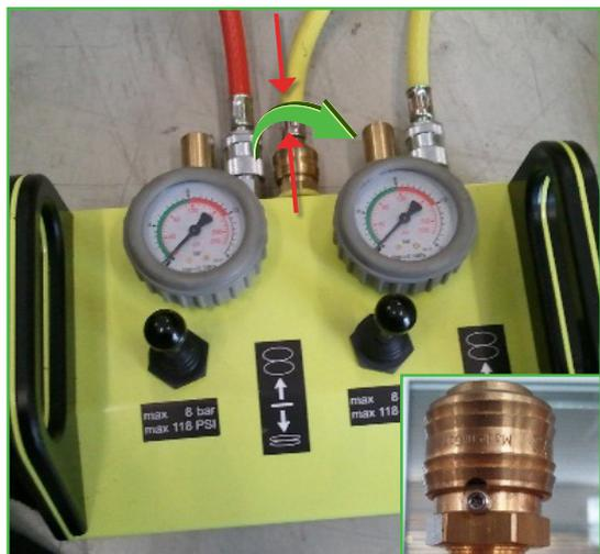
Turn the coupling housing until the groove on the housing clicks in, see Fig. 5.12 bottom right. Press the coupling housing toward the controller and pull out the hose connector.
