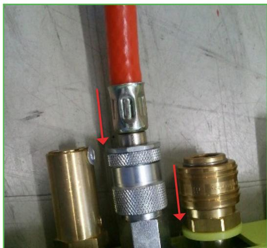
Insert the hose connector into the plug towards the controller. Press the coupling housing towards the controller. Release the hose connector to release it automatically from the coupling.
