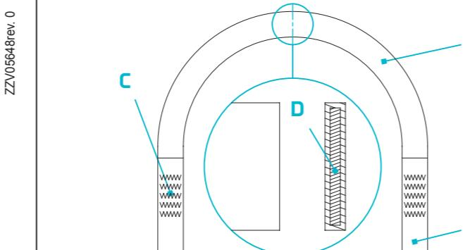
**EN:** (A) Tape, (B) Main stitch, (C) Internal wear indicator.
