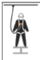
Fall Arrest Attachment Point Back "D"-Ring marked "A"
