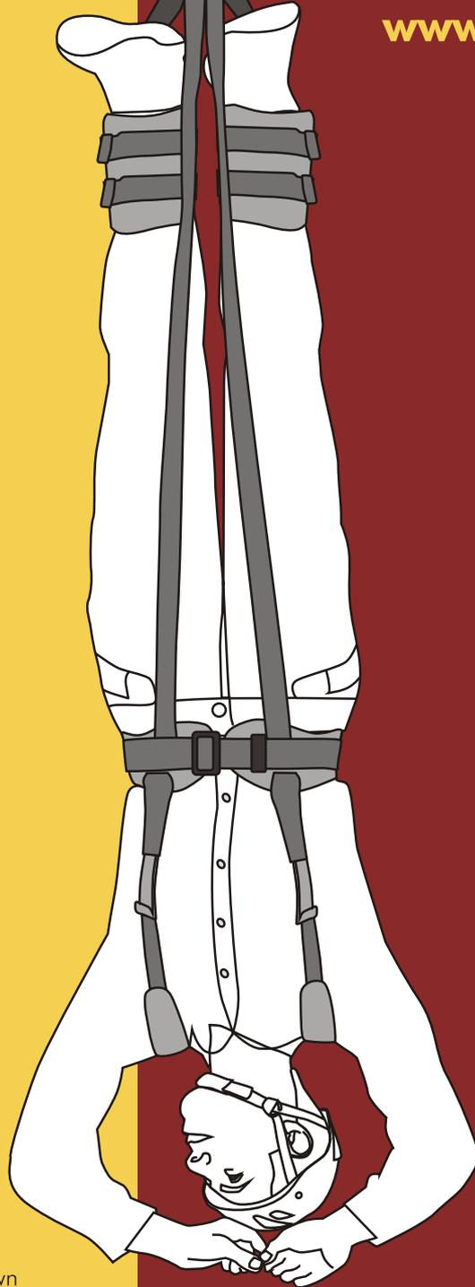
Special harness with ankle supports that allows head-down abseil in narrow spaces and tunnels (wells, silos, etc...). The high strength tape with strong stitches assures the max safety and reliability. The ergonomic paddings makes comfortable the overturned position, splitting the user's weight on shoulders, waist and ankles. Universal size with self-locking buckles easy to adjust. Accessory: special bag for material and tools to be hung to shoulder harness. Conform to EN 1498/C standards.
